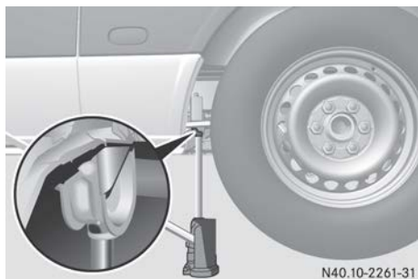
Jacking point, rear axle (example: panel van and crewbus up to 3.8 t)
