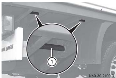
Lashing points: (example: platform truck)
