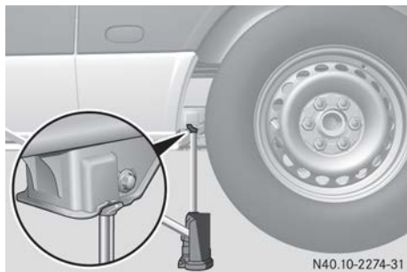
Jacking point, rear axle (example: panel van and crewbus, 5 t)
